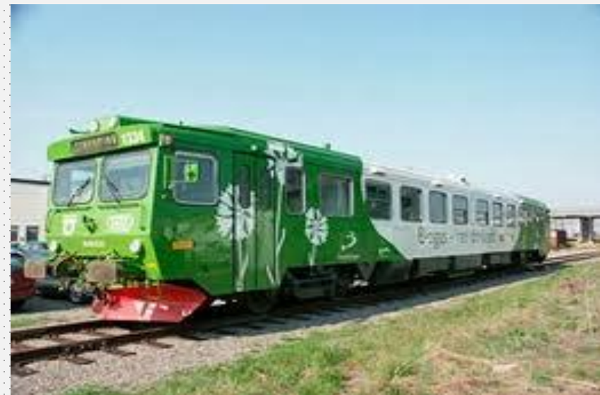
Biogas Train in Sweden
